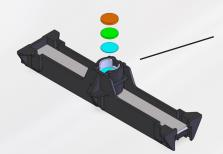
**Step 3:** Select the correct disks according to the pressure you need (depends on processed materials and cot shortens) and put the disks in the SpringUnit® (see table page 7).
